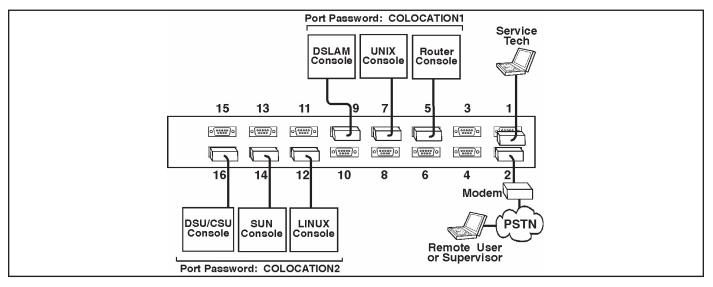
Figure 4.2: APS Application Example (Model APS-16 Shown)
